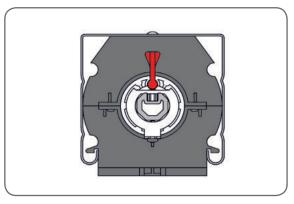
3. If the bottom rail is still not level, adjust it by changing setting of the pin in the mechanism to which the longest strap is attached.
