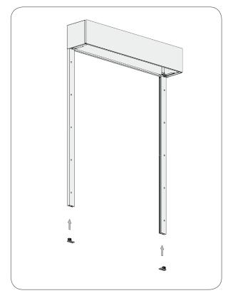
b) Position the guide channels and check the perpendicularity.
