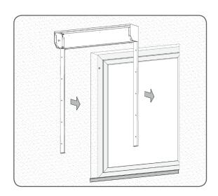
The roller shutter can be screwed directly to the window or to the wall.
