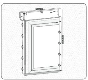
\_\_\_\_\_\_ Depending on the drive type used, before installing the roller shutter, determine the place where the tape, rope, crank or cable of the electric motor will exit
