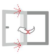
Do not turn the handles beyond their defined direction and range of rotation, as this could damage the hardware.
