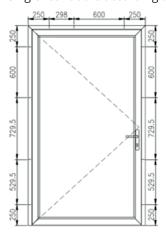
The maximum permissible fastener spacing for aluminium structures is 600 mm, with the distance between the outermost mounting elements and the corners being at most 250 mm.
