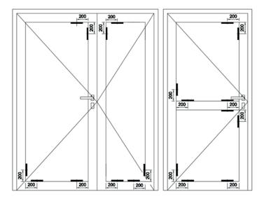
After correctly pushing out the door leafs, proceed to check the gaps around the perimeter between the door frame and the door leafs.
