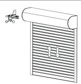
The Roller Shutter starts moving to a specific position and/or in response to the sensed weather conditions without any need for the user to interact with the controls. The user may, depending on the actual conditions, operate the key switch / portable transmitter.
